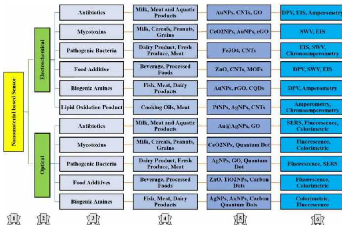
Fig. 2. Overview of Nanoparticle-Based Sensors for Food Safety Applications. The figure is structured as follows: (1) Nanoparticle-Based Sensor (main title), (2) Sensor Type (Electrochemical or Optical), (3) Analyte (e.g., Antibiotics, Mycotoxins, Pathogenic Bacteria, Food Additives, Biogenic Amines, Lipid Oxidation Products), (4) Sample (e.g., Milk, Meat, Aquatic Products, Cereals, Beverages, Cooking Oils), (5) Nanomaterial (e.g., AuNPs: Gold Nanoparticles, AgNPs: Silver Nanoparticles, CNTs: Carbon Nanotubes, rGO: Reduced Graphene Oxide, CeO 2 NPs: Cerium Oxide Nanoparticles, MOFs: Metal-Organic Frameworks), and (6) Technique Used (Electrochemical Techniques: DPV - Differential Pulse Voltammetry, EIS - Electrochemical Impedance Spectroscopy, SWV - Square Wave Voltammetry; Optical Techniques: SERS - Surface-Enhanced Raman Spectroscopy, Fluorescence, Colorimetric)
