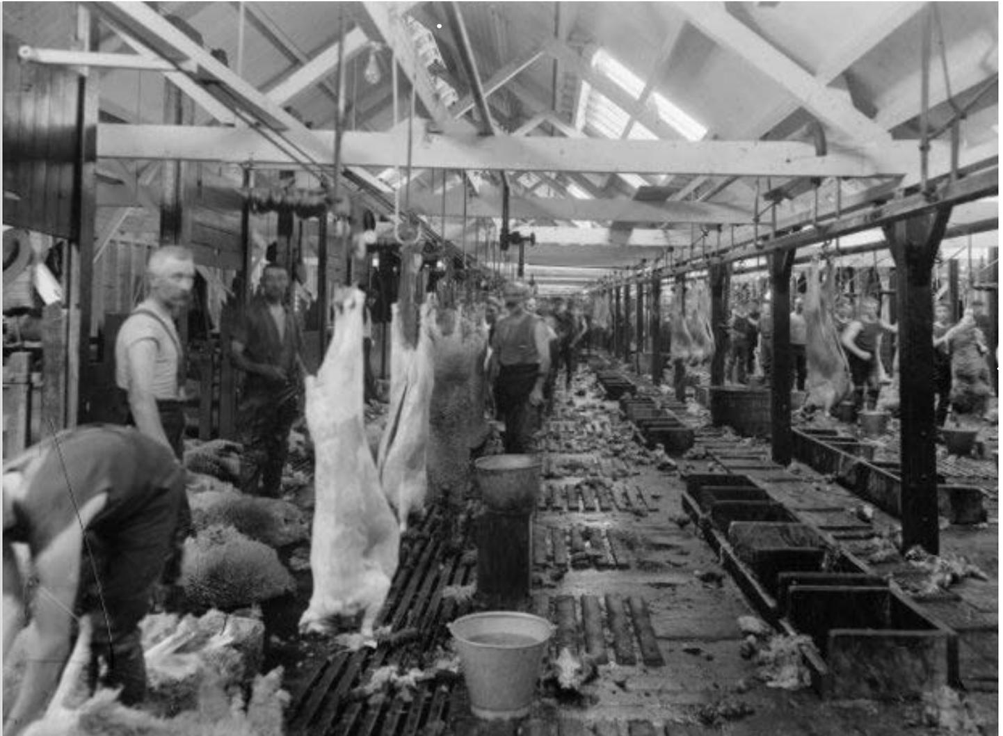
*The solo butcher system. Each butcher was allocated a bucket of water which had to last most of the day, and shared a laborer who ‘cleaned up’ and placed stuff in the holes in front of the butcher.*
